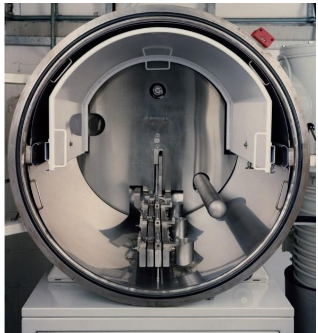
Identicoat 750 chamber interior with the evidence holder in the 'loaded' position. Three banks of metal evaporation sources plus the chamber lighting system are shown in the centre. The cryo 'cold finger' is shown on the right.
