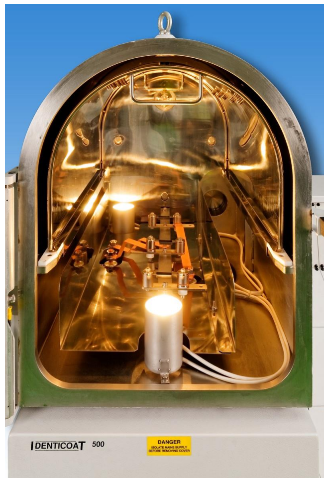
Chamber interior with the sample holder in place, showing the metal deposition sources and the chamber lighting system.
