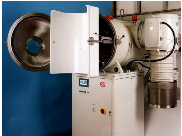
Identicoat 750 evidence holder in the 90-degree position. The holder can be completely inverted for particular evidence.
